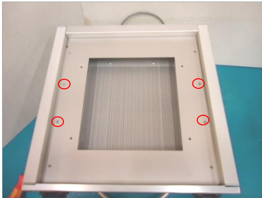
Figure 7. Remove Screws from Light Shield Top Cover
