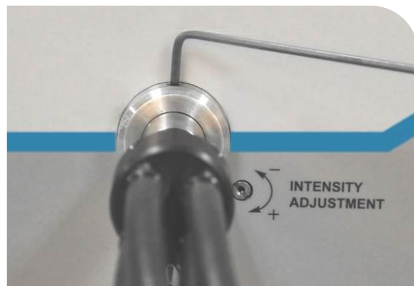
Figure 7. Gently Tighten Setscrew on Lightguide Mount with Hex Wrench
