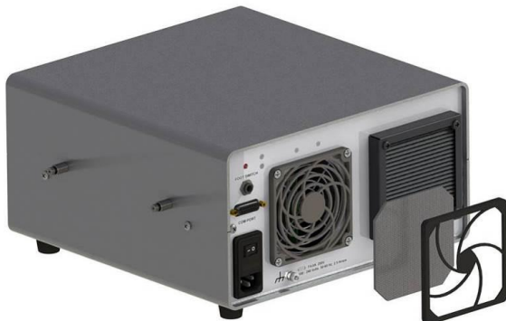
Figure 45. Intake Fan with Fan Filter Removed
