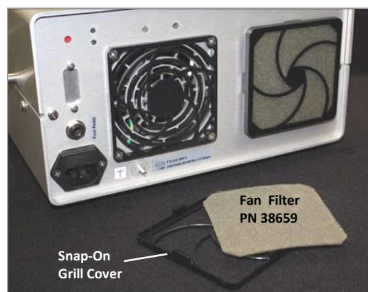
Figure 15. Fan Filter Replacement
