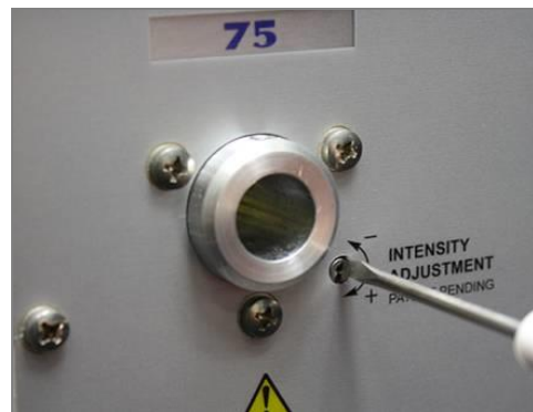
Figure 8. Adjusting Intensity with a Screwdriver
