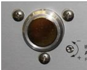
Figure 5. Shipping Cap in Lightguide Mount
