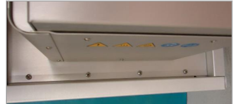
Figure 5. Connect the Lamp/Top Cover Assembly to the Light Shield by reinstalling the eight M4 x 8 mm Screws
